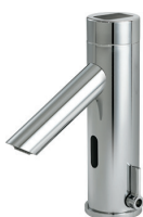
SOLAR ELECTRONIC LAVATORY FAUCET DEMD-321LF With integrated mixing valve and side mixer to adjust temperature 0.5 gpm (1.9 L/min)
